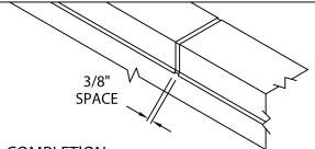
STEP 10 - COMPLETION CONTINUE INSTALLING COPING WITH A 3/8" SPACE AT SPLICE JOINTS TO ALLOW FOR THERMAL EXPANSION. FIELD CUT WHERE NECESSARY USING FINE TOOTH HACKSAW OR SNIPS. NOTE: REMOVE PROTECTIVE FILM IMMEDIATELY.
