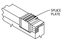
STEP 8 - SPLICE PLATES PLACE SPLICE PLATE ONTO ANCHOR CLIPS AT SPLICE JOINTS, 12'-0" O.C. NOTE: REMOVE RELEASE PAPER FROM SEALANT STRIPS.
